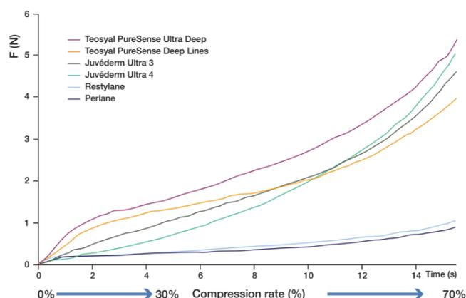
Figure 2 shows, for different fillers, the force required in order to flatten the gel with a linear increasing degree of compression from 0 to 70%. The curves allow to distinguish two types of materials:
